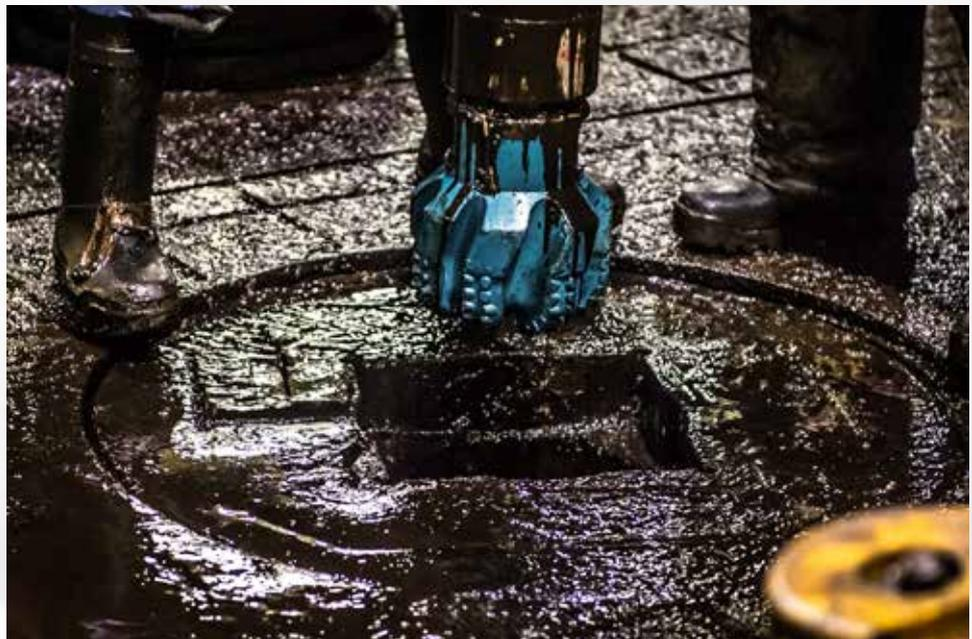
**Figure 2.** Ulterra's PDC drill bit going into the hole is the final step of the product development system.
