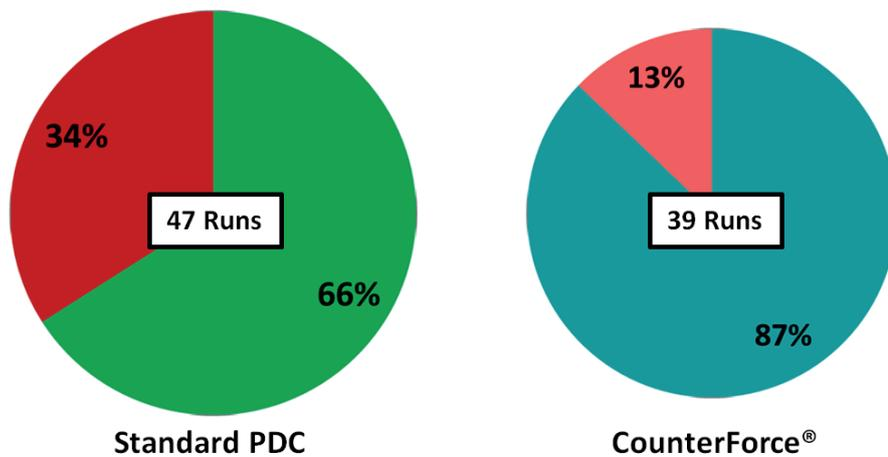
**Figure 3.** The percentage of RSS runs pulled for downhole tool failure. Rotary Steerable tool reliability has positively correlated with the use of CounterForce bit technology over a statistically significant data set.
