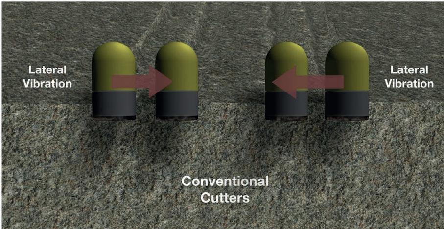
**Figure 1.** Traditional PDC cutting structures are laid out to be balanced, or neutral to drilling vibrations.
